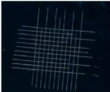
Adhesion tests of Parylene on Silicon after 1 \cdot 10^{16} neutrons \text{cm}^{-2} (nucl. reactor irradiation)
