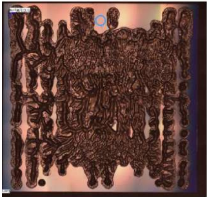
Glue pattern after using the final prototype stencil: continuous glue layer
