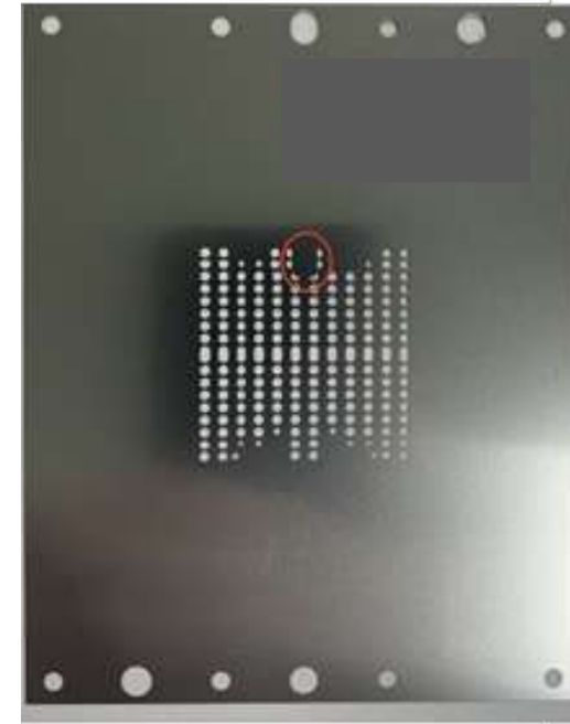
Stencil >80\% glue coverage after compression
