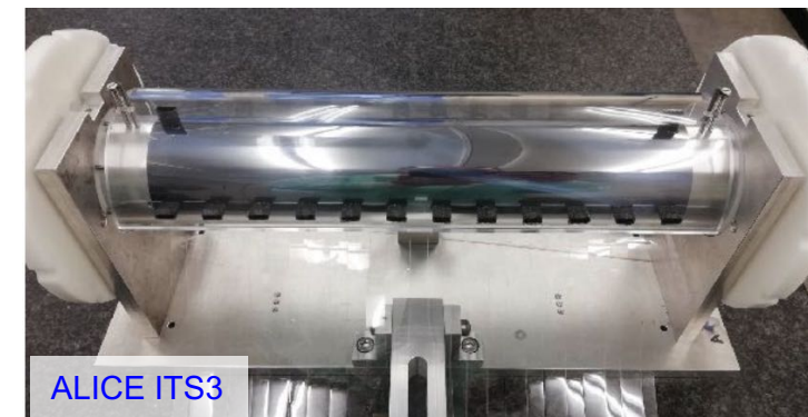
Bent wafer-scale dummy sensor on foam support
