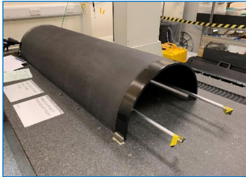
Prototype Outer End-cap shell and associated metrology results
