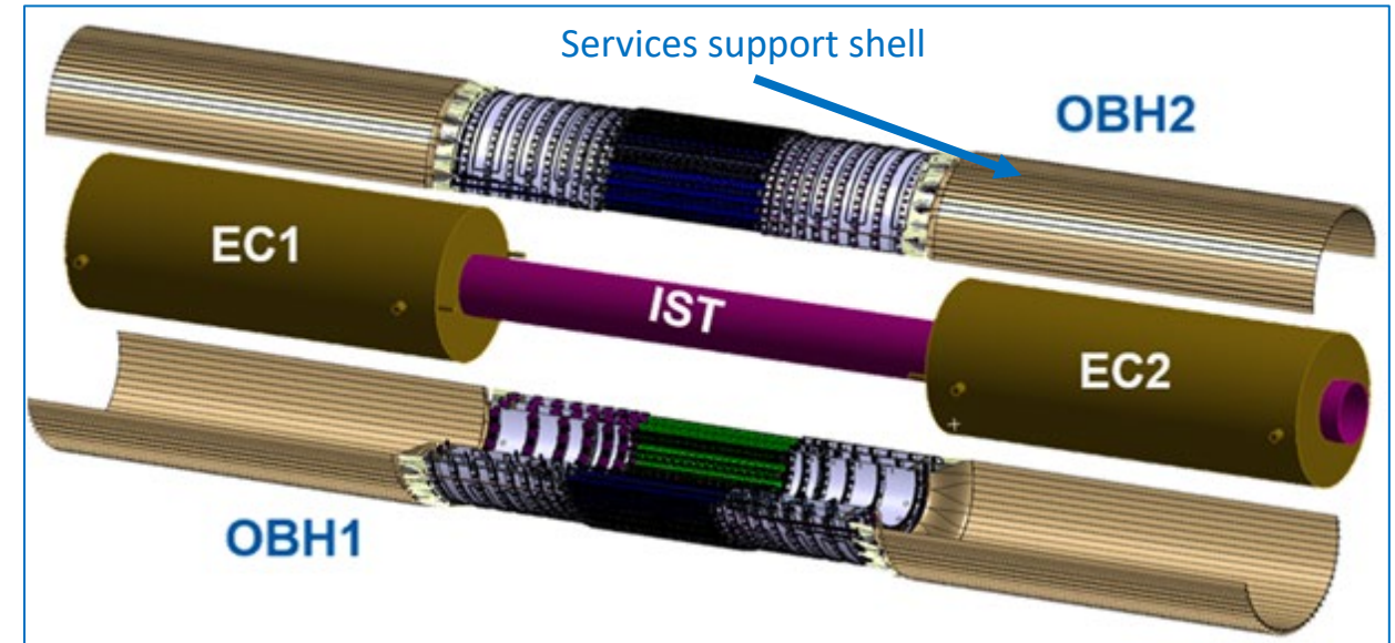
Integrated outer system (exploded view) showing the outer barrel services support shells
