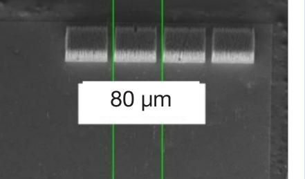
Segmented VACNTs bumps [yap] VACNTs could be used as the detector substrate or, in the case of hybrid detectors, as a pixelated interposer between the ASIC and the sensor as illustrated below.
