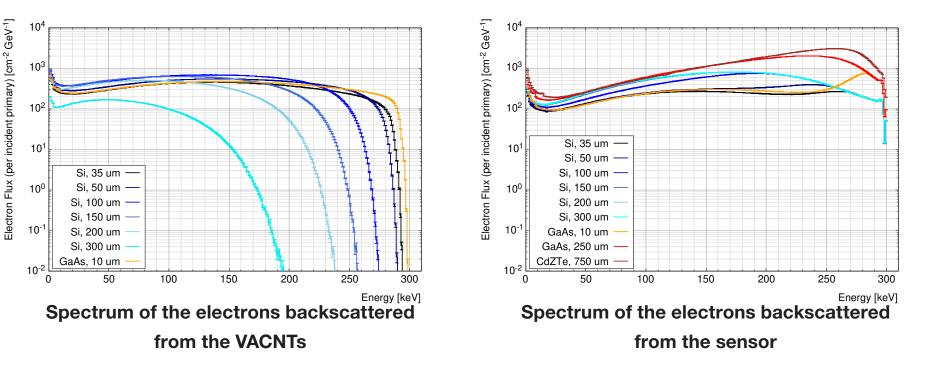
The DQE is also affected by the fraction of the primary beam which is directly bouncing off the sensor surface (with or without prior interaction). This effect is stronger for high-Z material such as CdTe or CZT although the reduction of the thickness help to minimize its effects. Although this has nothing to do with the detector substrate, it's worth mentioning that sensor thicknesses above 150 um will only have limited benefits from the mitigation
