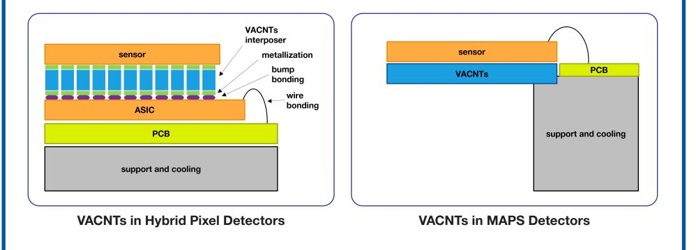
In both cases the VACNT layer would assure an optimal heat extraction channel when coupled with an active cooling system. A decrease in the intensity of the direct backscattering radiation (photon and/or electrons) entering the detector from the back would be also granted by the low atomic number of carbon.
