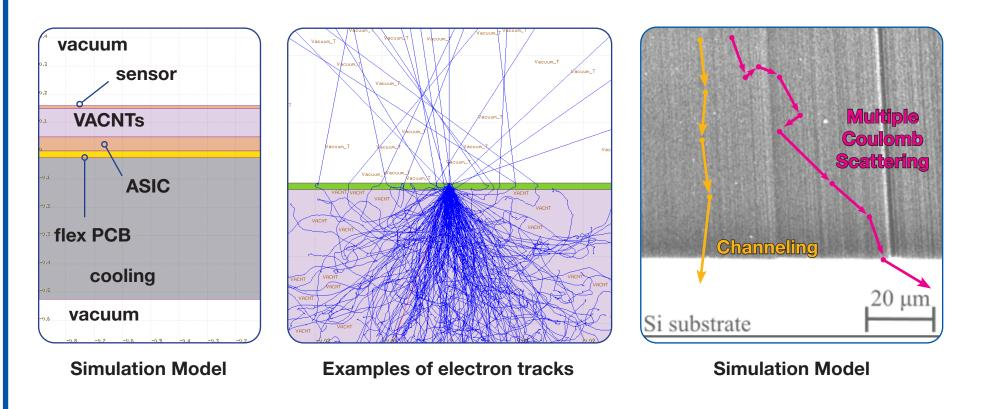
The selected sensor configurations used for this study were: • Si (thicknesses: 35, 50, 100, 150, 200 and 300 µm); • GaAs (thicknesses: 10 µm and 250 µm); • CdTe (thickness: 750 µm).
