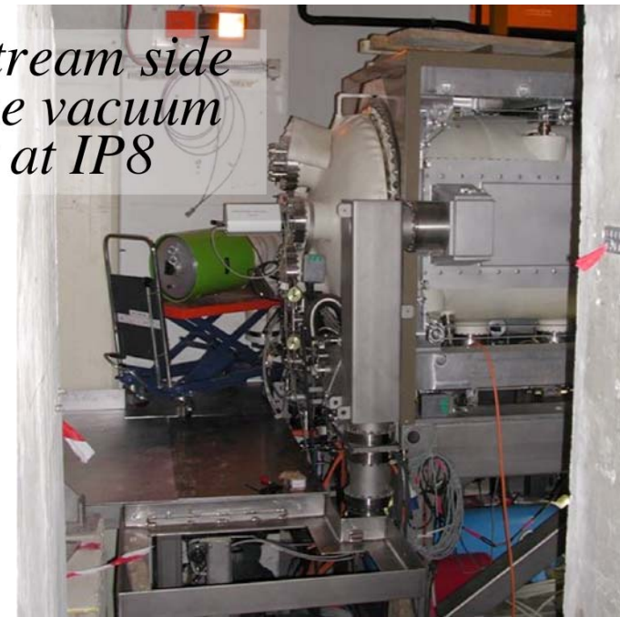
Al window and wake field suppressor
