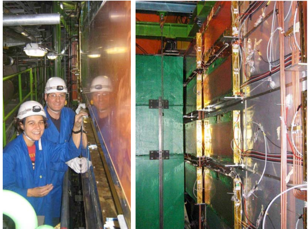
MWPC installation for M5
