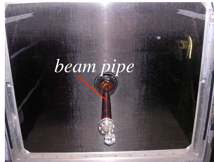
RICH-1 exit window
