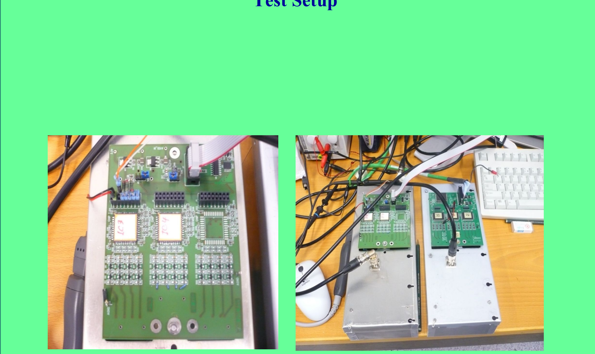
New Mezzanine card (2-layer PCB) with new 2xASD mounted side-by-side comparison of previous chip/card and new
