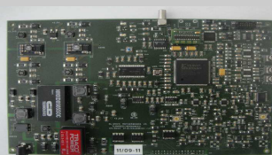
Alibava mother board used in the telescope with the readout bus terminator
