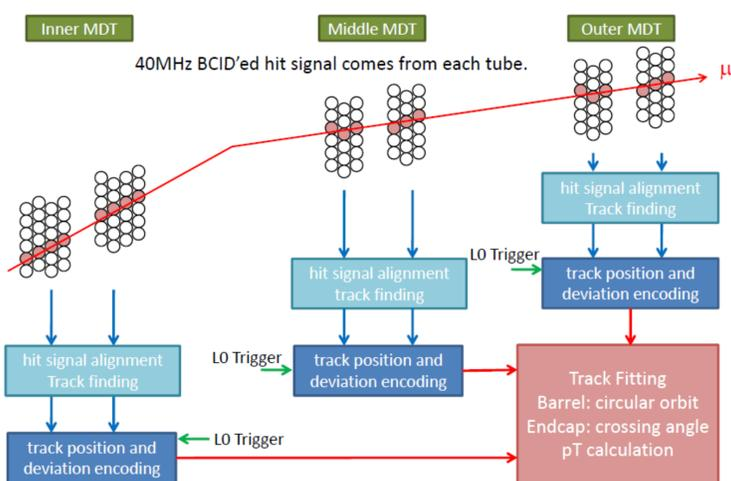
The signals from all the MDT tubes are BCID'ed with 40 MHz LHC clock and sent to the counting room. The straight-line track finding in each MDT station is made in parallel. The outputs from the finding are information about the track position and its deviation from the infinite  $p_T$  track. The Level-0 signals from TGC and RPC will assist the track finding. The track information from each stations is combined and the  $p_T$  momentum is calculated.
