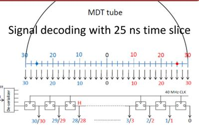
Spatial-aligned hit signals at 40 degree incidence
