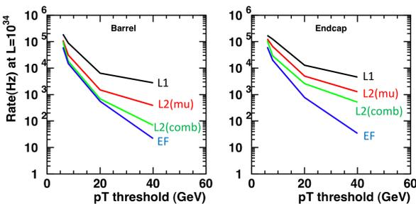
The figures show the simulated trigger rates of Level-1, Level-2 and Event Filter (EF) at  $L=10^{34} \text{ cm}^{-2}\text{s}^{-1}$ .
