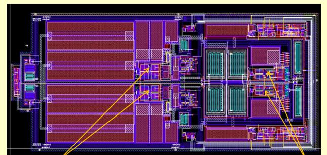
Integrators Dual-Ramp Generator Layout Mirror sources
