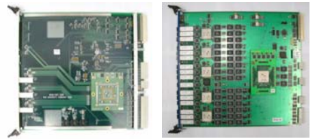
Muon Port Card with old Virtex-E mezzanine (left) and Sector Processor (right)
