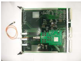
Muon Port Card with the new Virtex-5 FPGA mezzanine
