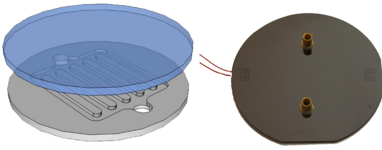
One option, the gas cooling, consists of a vessel with Kapton windows on both sides of the detector placed inside the beam vacuum where a gaseous nitrogen flow ensures the cooling. The nitrogen will enter the vessel at a temperature of 100 K. The cold flow will keep the operation temperature of the module less than 5°C. The total thickness of the Kapton foils is 100  $\mu$ m.
