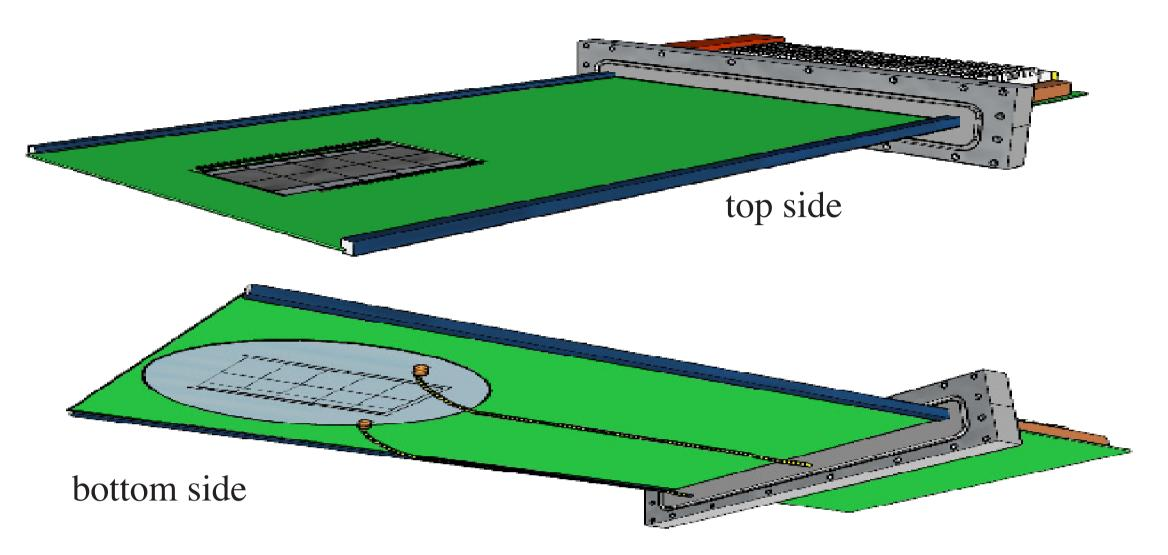
The assembly carrier holds the sensor-pixel ASIC assembly and references it precisely in place, provides electrical connections to the detector electronics for power, control and the high speed Gigabit electrical transmission lines and provides the mechanical interface between the detector assembly and the cooling. The design is compatible with both cooling options.
