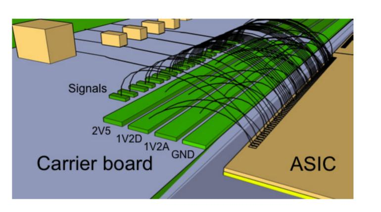
Wire bonds provide the electrical connections between the ASICs, the sensor and the GTK assembly carrier. In order to avoid the need of a precise pitch adapter to the printed circuit board, a staggered wire bonding scheme is proposed where the pitch in the PCB is larger than the ASIC pad pitch of 73  $\mu$ m.
