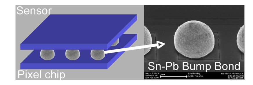
The sensor of 200  $\mu$ m thickness is bump bonded to the read-out ASICs, thinned to 100  $\mu$ m. Sn-Pb or Sn-Ag bump Bonds will be used.
