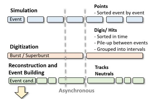
Data synchronous from reco. level passed to software trigger and analysis
