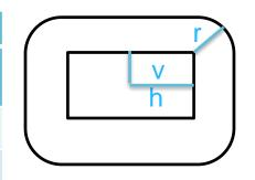
(1) Displacement of the aperture and the actual orbit due the combined effects of alignment position and orbit leakage.
