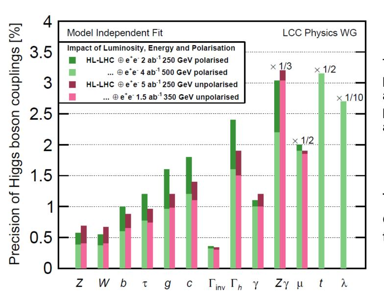
There are no drastic difference between precision with 2 ab<sup>-1</sup>, polarized beam and precision with 5 ab<sup>-1</sup>, unpolarized beam at 250 GeV.
