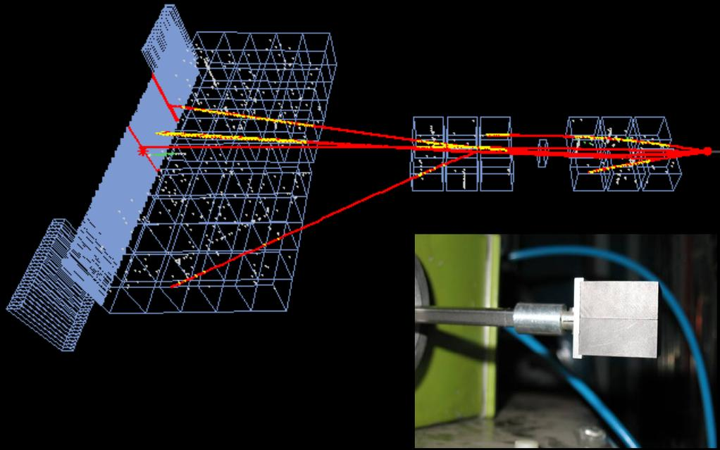
**p+(T2K replica target) at 31 GeV/c**
