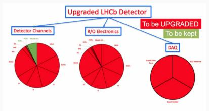
Less than 10% of detector channels will be kept 100% of R/O electronics will be replaced
