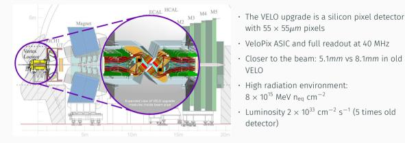
$\cdot\,$  Modules operate in vacuum, separated from LHC vacuum by RF foil
