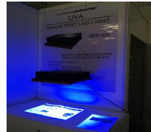
CRACK TEST UV-365nm
