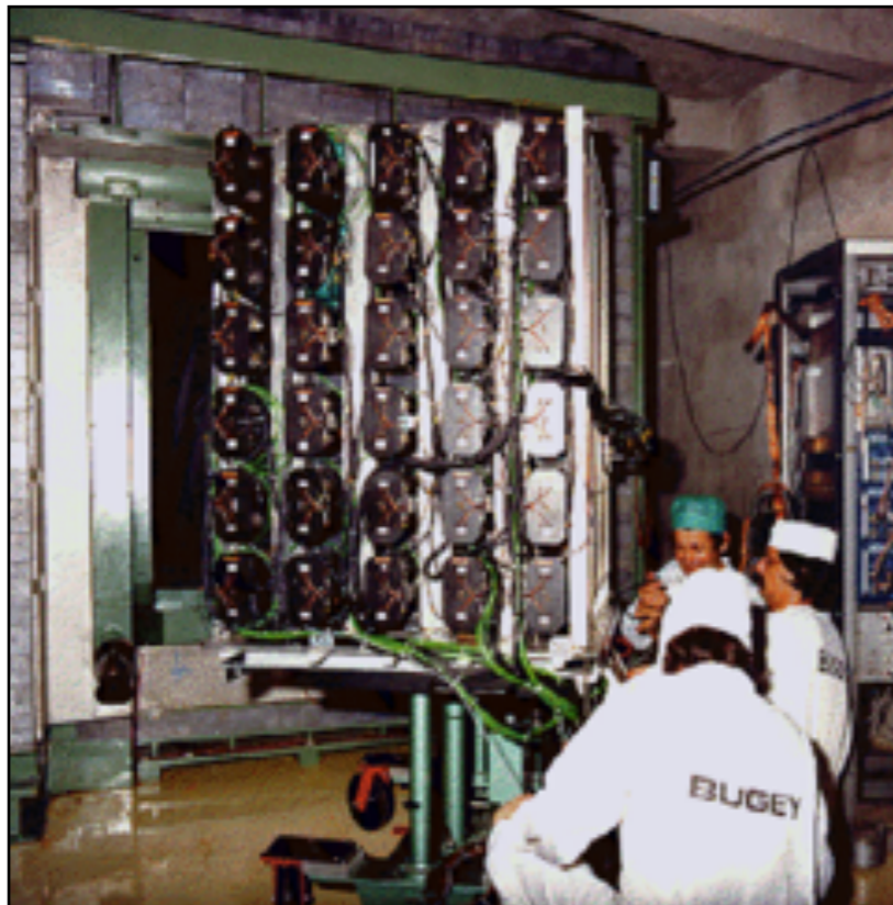
1980s: Bugey: ~1000 counts per day, S:B 10:1, but only underground. flammable/corrosive solvent detector liquids
