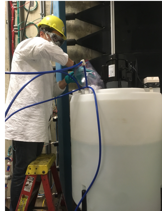
Gd-loaded water filtration
