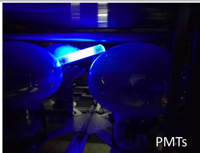
TPB coated glass on top of THGEM
