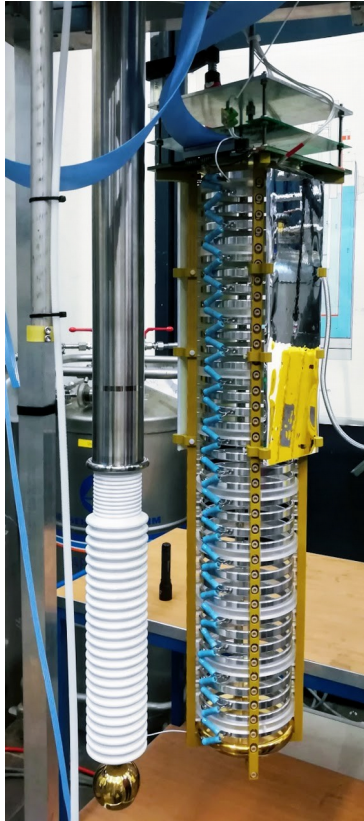
60 cm drift test TPC, prototype pixel anode, and unfiltered 3D information from a cosmic muon. JINST 13 (2018) no.10, P10007.
