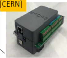
Figure 2: Scavellone detector. The portable, standalone version of the MoCoS device is housed in a 3U format case and has to be connected through all around the device.
