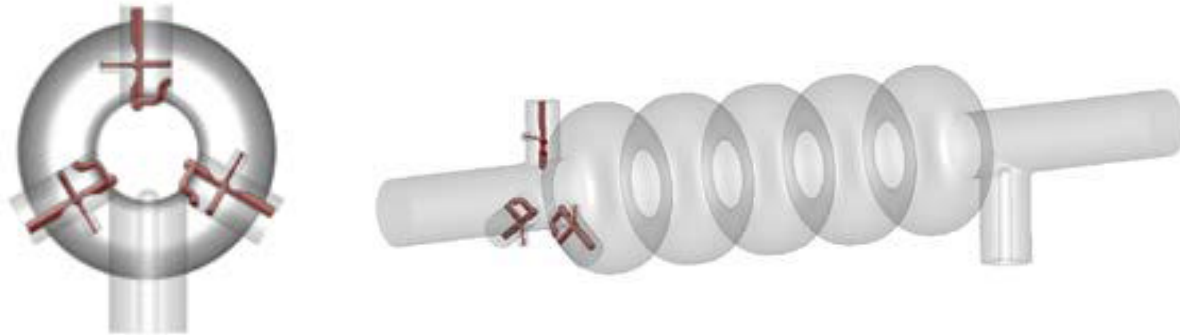
Scaled DESY/TESLA-type HOM couplers with Y configuration
