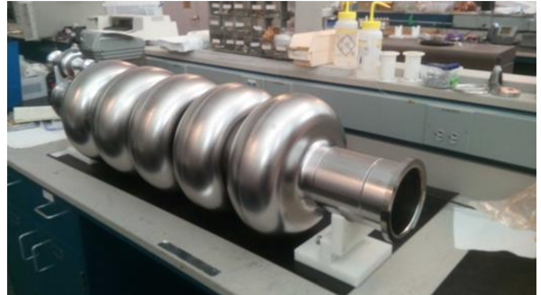
The first Nb 802 MHz 5-Cell cavity fabricated October 2017 at JLAB
