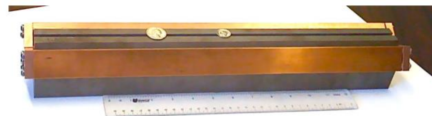
Fig. 6. Electro-magnets with a small 5 mm gap prototyped for the eRHIC linac-ring design and tested at 0.43 T [9-10]. FCC ee needs dipoles with a magnetic field of up to 0.04 T and could be driven by a coil with low current.
