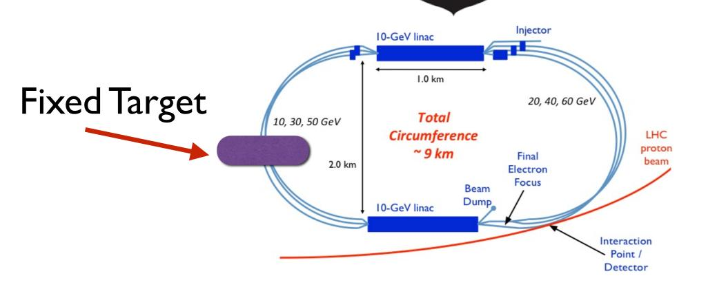
Use LHeC 60 GeV Electron Ring in Fixed-Target Mode
