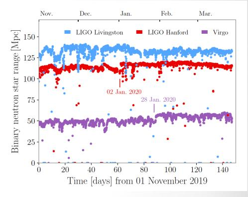
Measure of detector sensitivity: The binary neutron star range represents the distance a detector is able to detect a signal from a 1.4-1.4 solar mass binary
