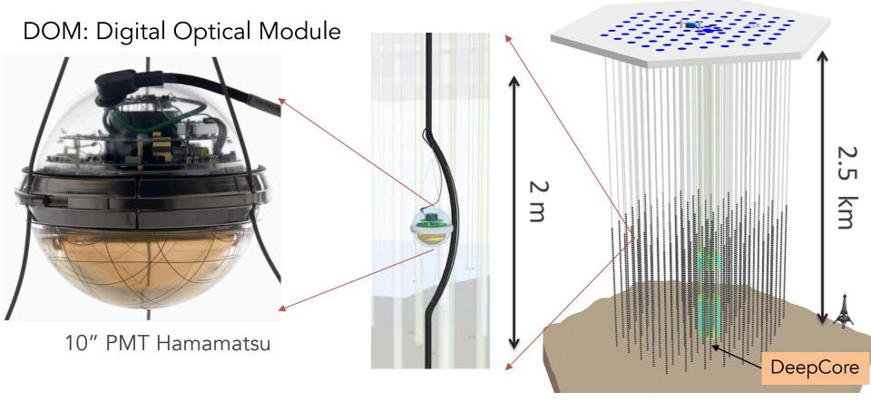
5160 DOMs spread over 1 km<sup>3</sup> = 1 Gigaton instrumented volume
