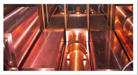
Residual contaminations in the new DAMA/LIBRA Nal(TI) detectors: <sup>232</sup>Th, <sup>238</sup>U and <sup>40</sup>K at level of 10<sup>-12</sup> g/g
