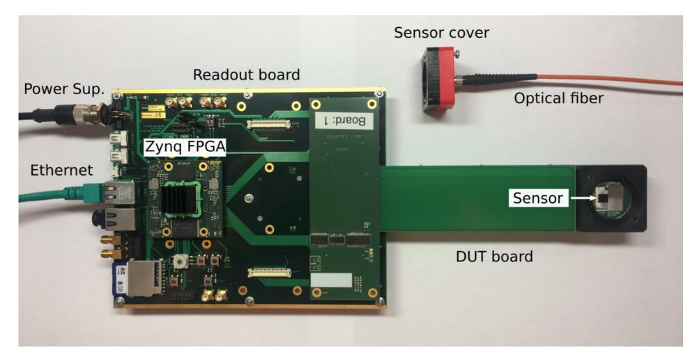
Simple mechanics, only supply voltage as analogue bias. FPGA for data collection.
