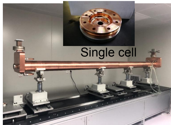
The accelerating structure under tuning
