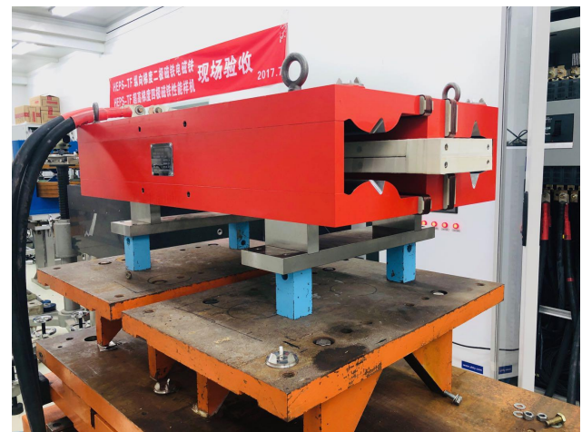
First dual aperture dipole test magnet of 1m long has been finished in Nov, 2019
