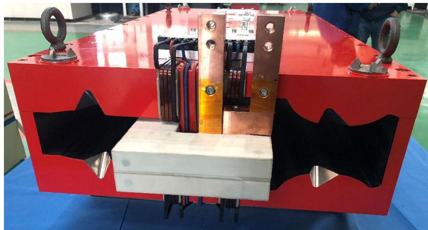
First dual aperture dipole test magnet of 1m long has been finished in Nov, 2019
