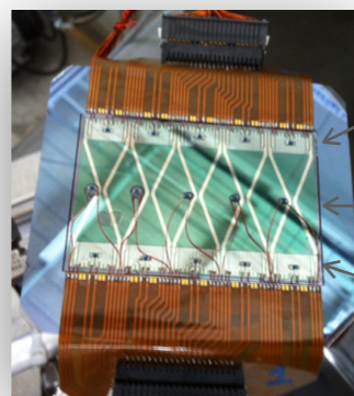
CP equipped with thermo-mechanical mockup of the hybrid detector
