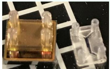
polymer fluidic channels 3D printed on the back of a working CMOS chip
