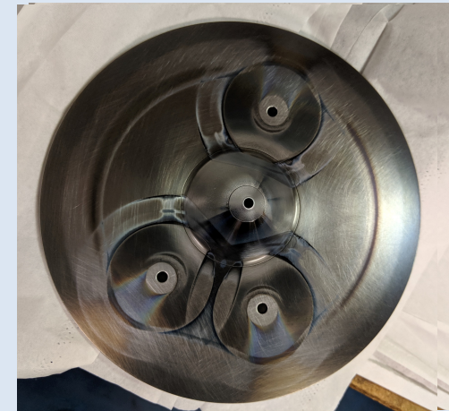
Ion source facing side of the extractor after 9 months operation does have cesium deposits
