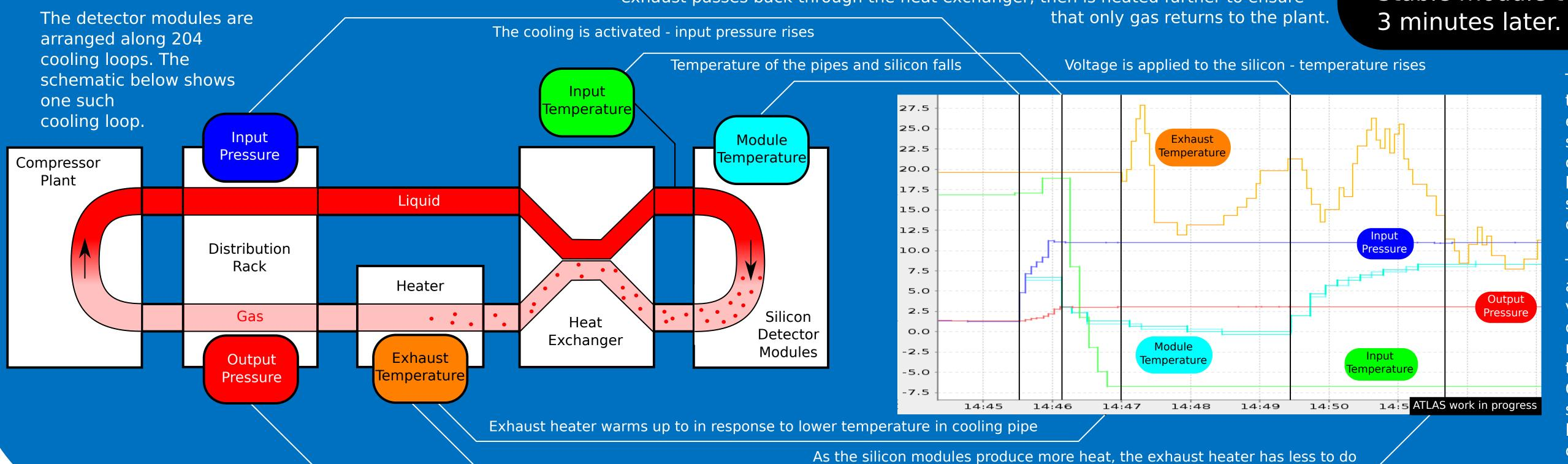
This plot [2] shows the sequence of events when switching on a cooling loop after it has had time to stabilise at ambient
