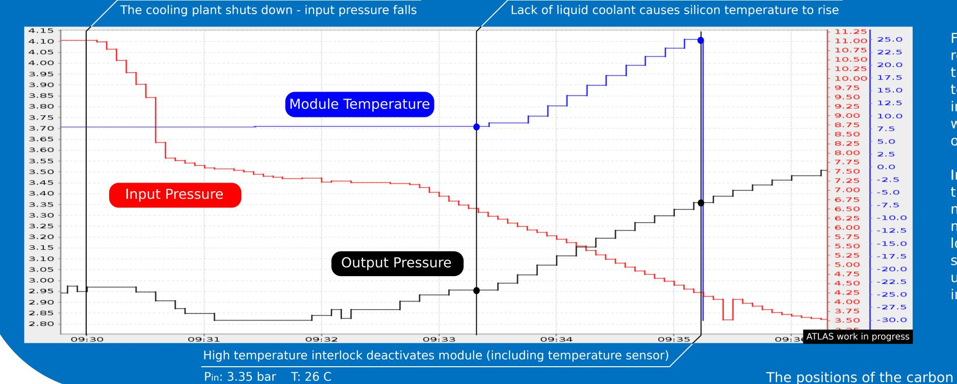
For 200 seconds the silicon temperature stayed constant as the remaining liquid coolant boiled off and the vapour pressure equalised throughout the exhaust system. Once this had finished the silicon temperature rose rapidly, going up 18 C in 2 minutes. Hardware interlocks were triggered by the high temperature and the modules were powered down automatically, protecting the detector from overheating: the detector was never at risk.
