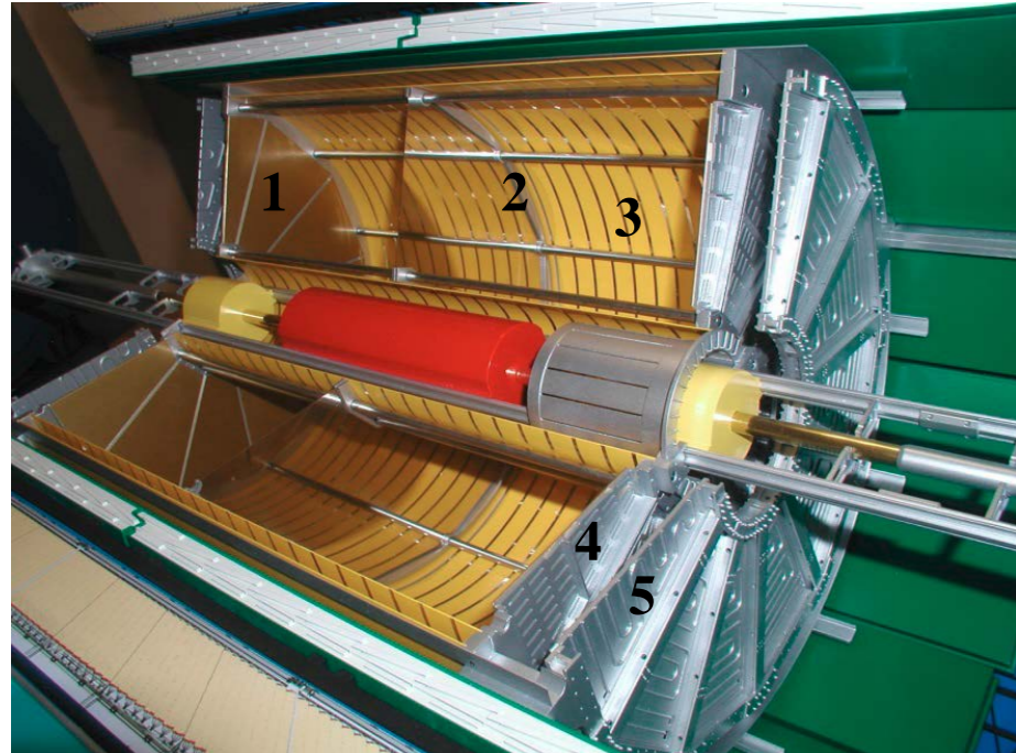
Central part of the MPD mock up with TPC cut
