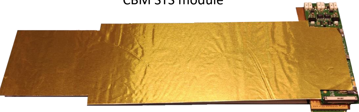
STS module covered with shielding
