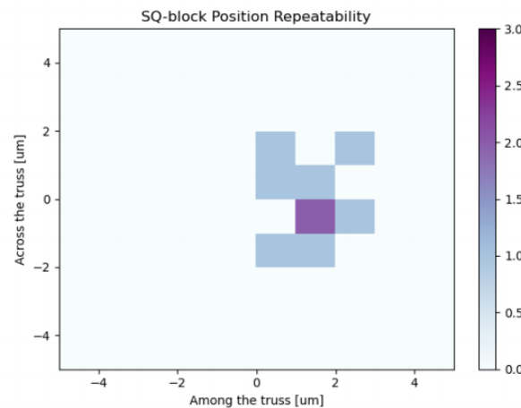
CF-truss position repeatability test
