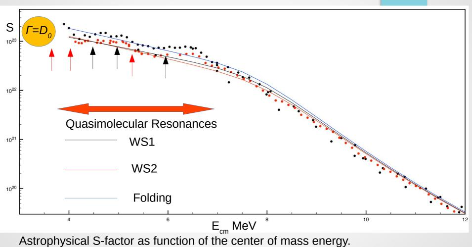
Points — experimental data.  $\Gamma=D_0$  — area where widths of the compound states are smaller than their average spacing. Red and black arrows are prediction of the resonances for N-1 band for WS1 and WS2 respectively.
