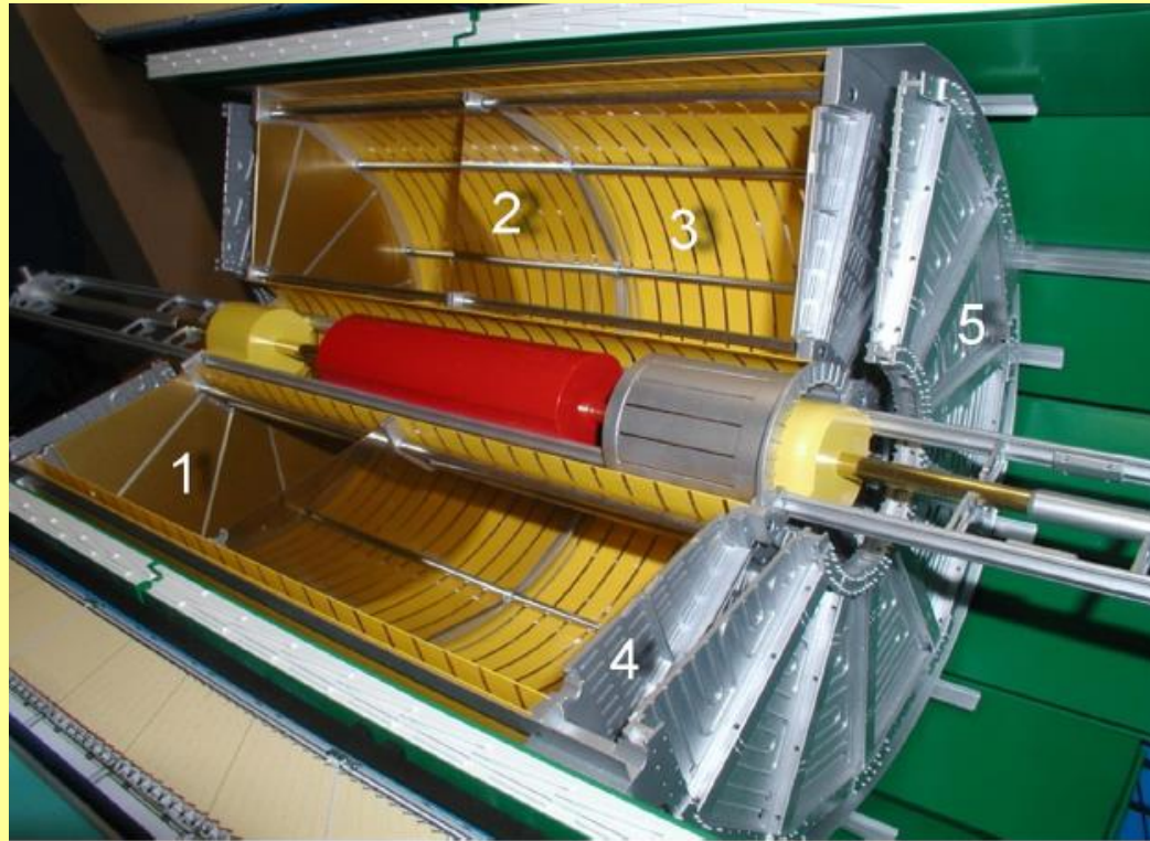
Time projection chamber for multi-purpose detector at NICA, Nucl. Instrum. Methods Phys. Res. A 958 (2020) 162793,
