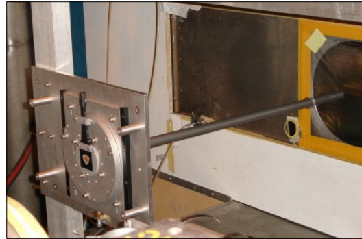
T2K replica target – 90 cm graphite rod
