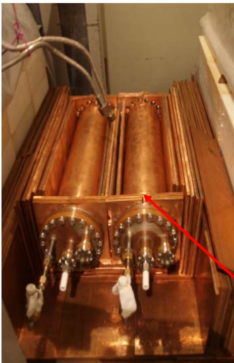
Two proportional Kr-chambers with the first layer of passive protection. Spectrum of the Kr camera measured over 613 days. Limits on g_{A\gamma} . Decay scheme and the Andyrchi mountain, under which the BNO INR is located at a depth of 4800 m.
