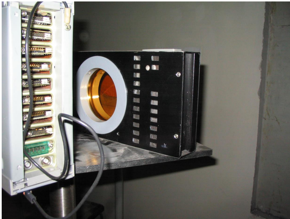
The multi-channel chamber is on the left, the narrow-gap chamber is on the right
