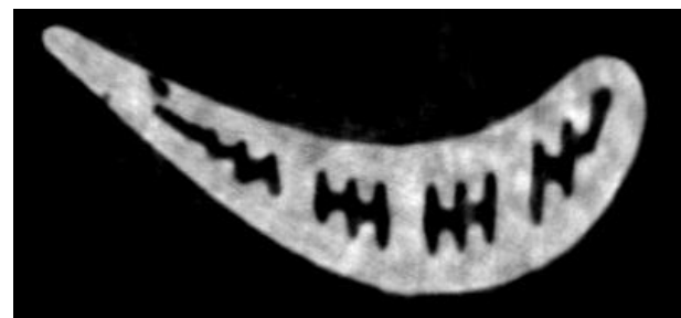
Neutron visualization of the parts of gas-turbine engine
