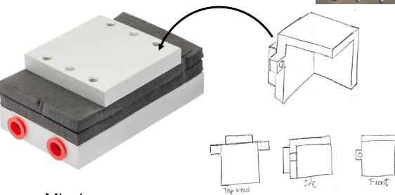
Creation of a cooling block sample holder compatible with edge/top injection
