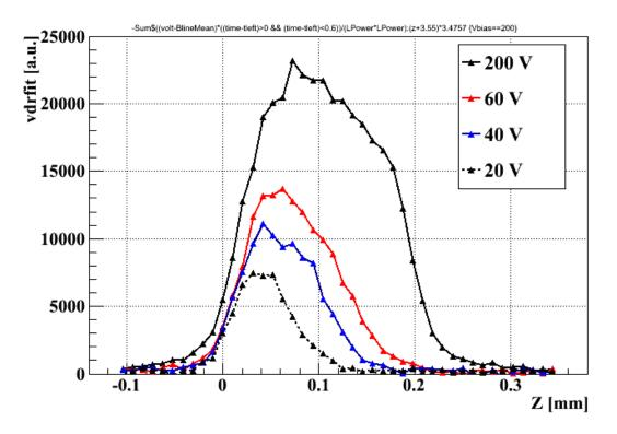
Voltage scan of HPK 200 µm thick detector Shown E-field calculated as a function of depth Detector (not irradiated) depletes from the front Depletion width increases with voltage This measurement can not be done with top/bottom SPA-TCT
