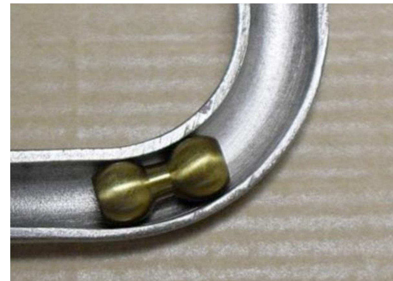
Dumb-bell-shaped capsule in a bent segment of the calibration tubes.
