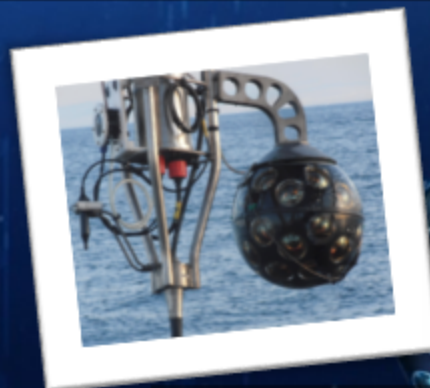
Test of photon counting capabilities and directional sensitivity of DOM. Eur. Phys. J. C (2014) 74:3056
