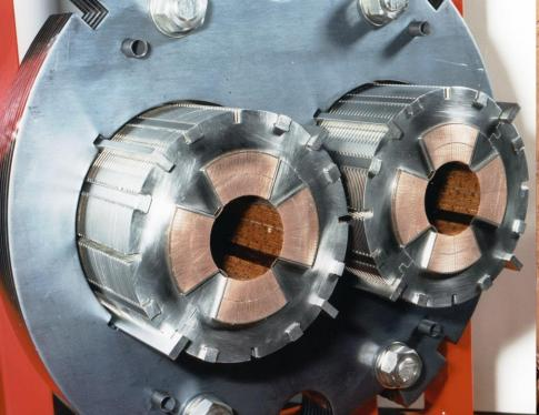
~ 400 quadrupole magnets focus the beams
