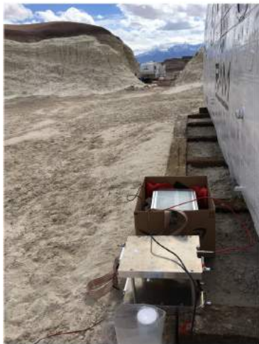
Two detector layers at the time of data-taking in MDRS
