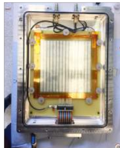
Detectors assembled with readout and high voltage electronics system
