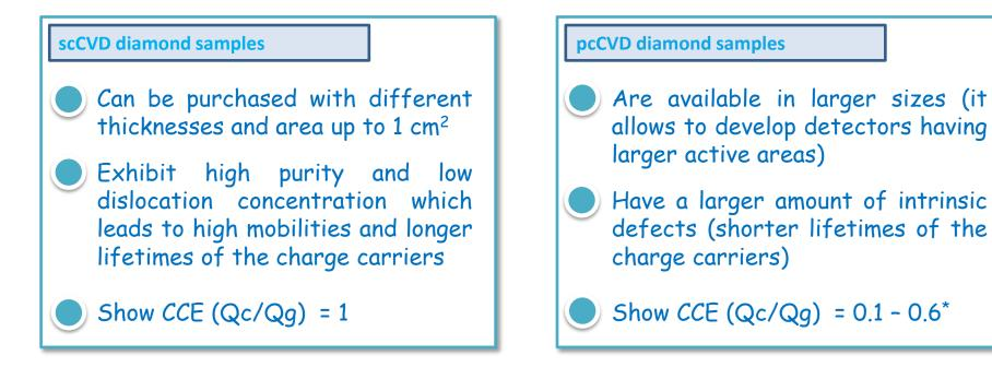
\*Particle intensity monitors based on pcCVD diamond samples may suffer from a reduction in their counting efficiency. Indeed, the partial CCE may generate signals having amplitudes below the threshold value of the discriminator.
