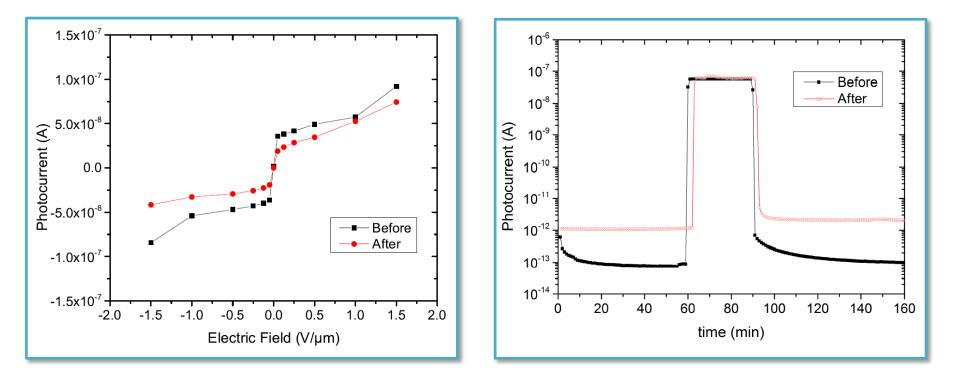
Long term measurements recorded with electric field applied of 1 V/µm
