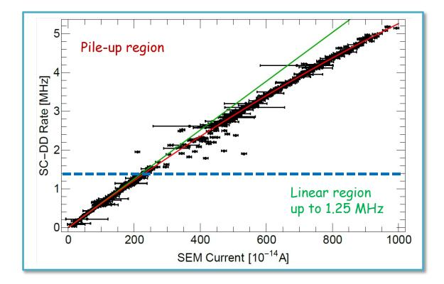
The calibration factor was found as linear parameter of a second order polynomial fit  $[K = (6295 \pm 320) \cdot 10^{14} \text{ ions/A}, \text{ uncertainty } \sim 5\%]$
