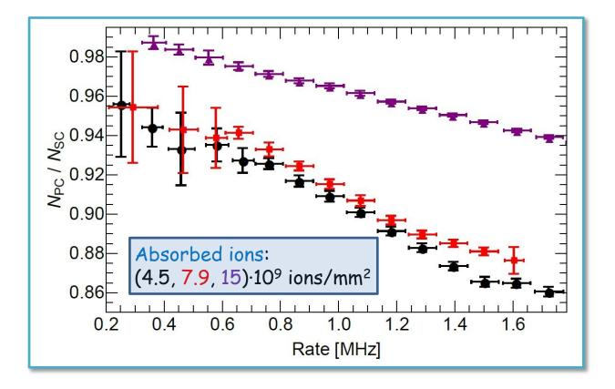
PC-DD Counting Efficiency [< 700 kHz<sup>\*</sup>]: (94.8 ± 2.5)%
