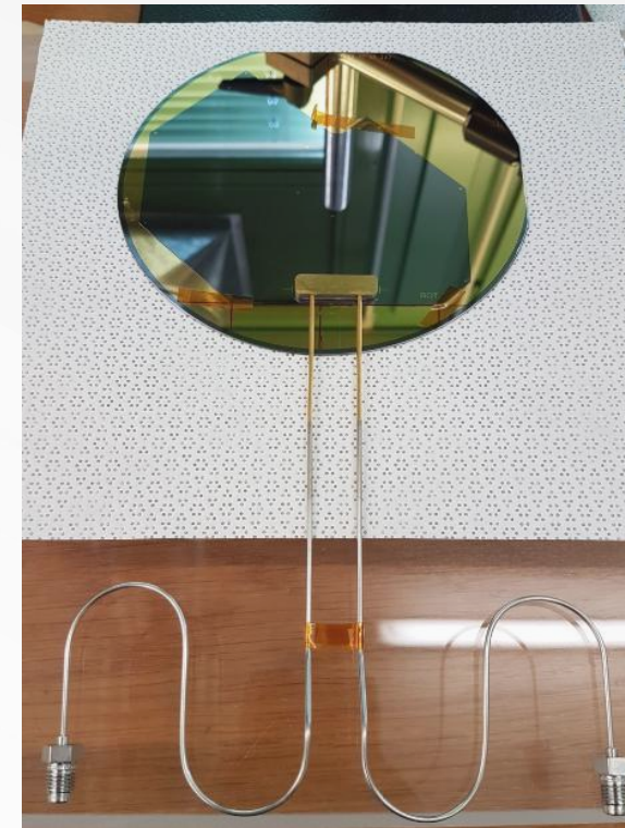
Soldered panel, cooling pipes are connected to micro-channel substrate
