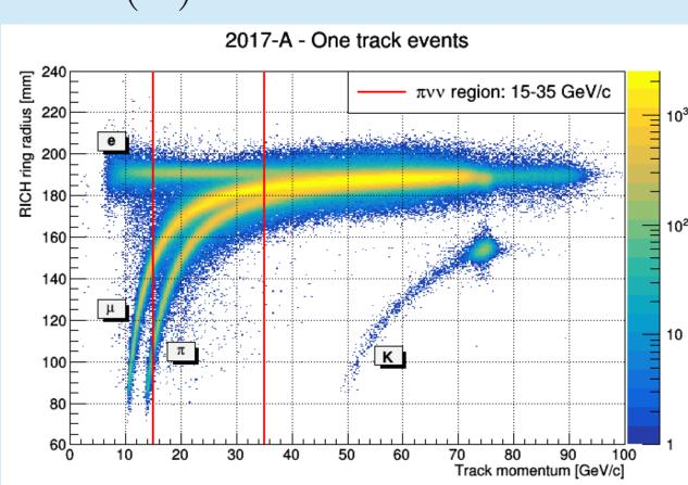
• Particle mass, m(R,P), reconstructed with RICH, for muons and pions in the momentum range 15-35 GeV/c:
